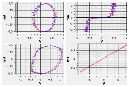
In the case of the ASA EyePoint, the analysis is based on comparison. This means comparing the signature of the reference (known to be working) printed circuit with the signature of the verified printed circuit (with suspicion of a malfunction). The difference in the received signatures may indicate that the tested schema is the source of a potential problem and may not meet the stated requirements.
