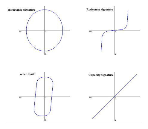
The signatures below were obtained by using the ASA EyePoint p10, EPC MSU. Some signatures were taken from actual tests of reference boards and non-working boards.
