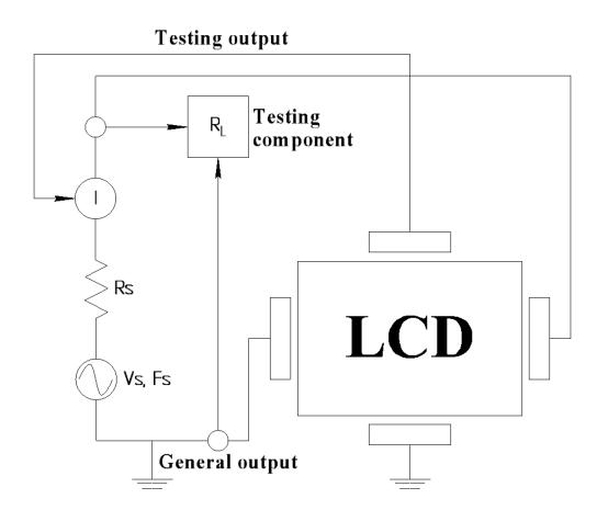
Rs - source resistance, Vs - source voltage,  $R_L$  - load resistance, Fs - signal frequency.
